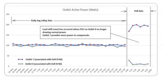
In this depiction of a load shift scenario, the left side is 30 days of daily rollup data and the right side is one hour of polled data taken every 10 minutes. Normally each power supply is using 100W to power the server. On the right, you can see that Outlet 8 has failed, and for the past hour the server has been running on just Outlet 7 which has had to increase its load to compensate.
